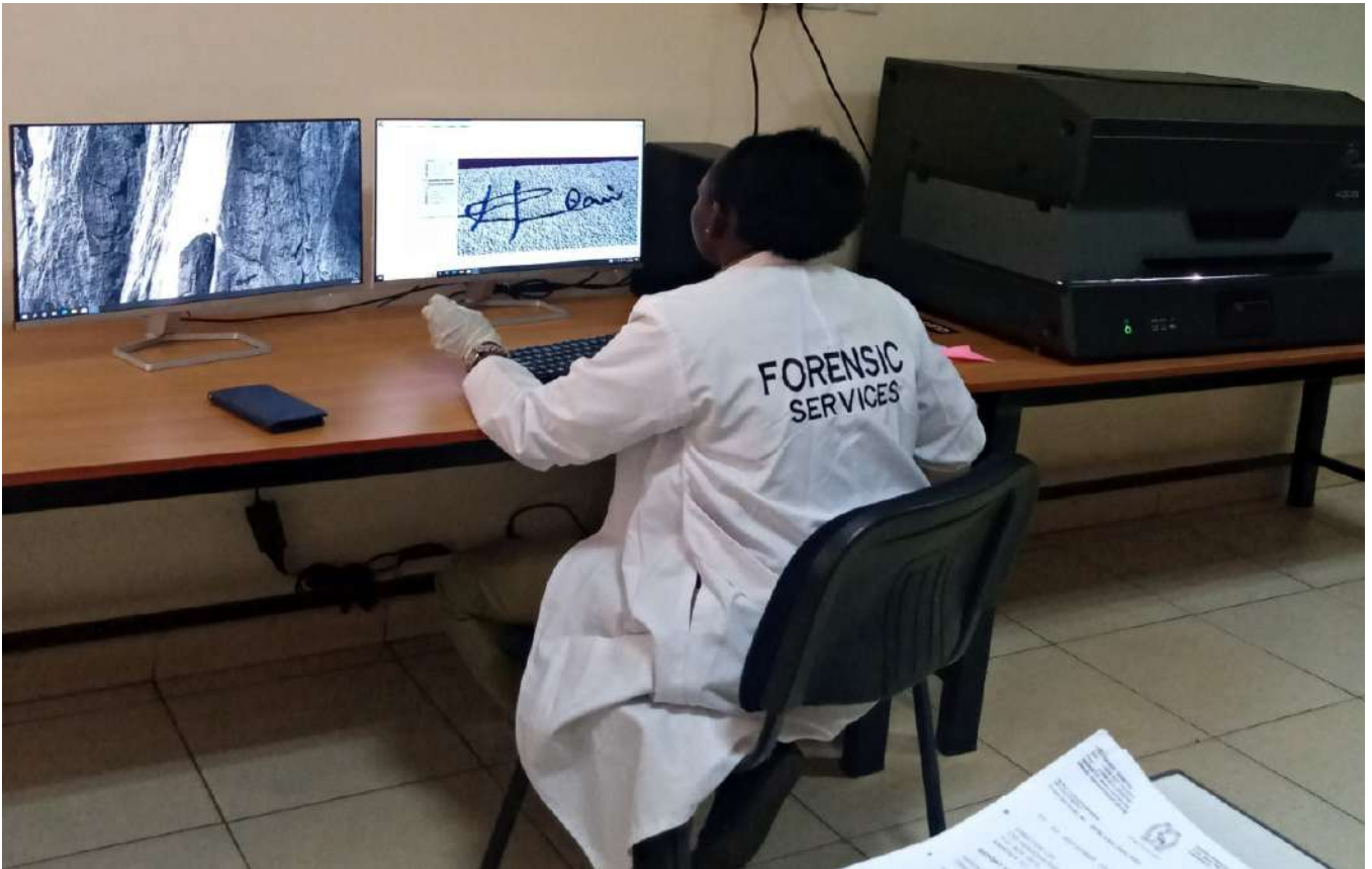
A forensic document examiner analysing a disputed signature on a Video Spectral Comparator
